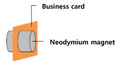
2. Measure and record the magnetic field values of the front and back sides of the joined magnets as shown in the diagram below.
